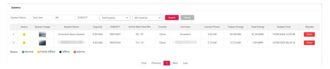
**Abnormal MPPTs:** the number of MPPTs that have alerts within the latest 15 minutes under the distributor account. **Total MPPTs:** total number of MPPTs with data uploaded within the latest 15 minutes.
